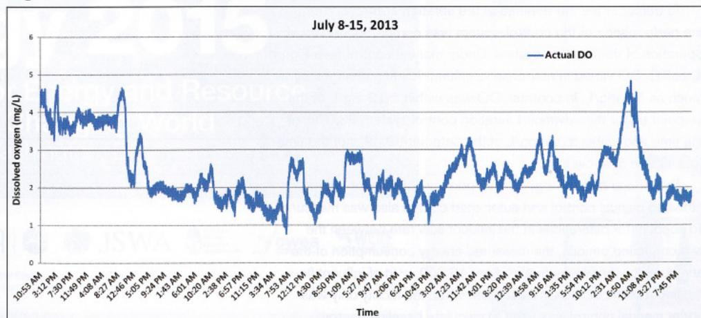
**Figure 5. DO levels during automatic-aeration control for 1 week**
